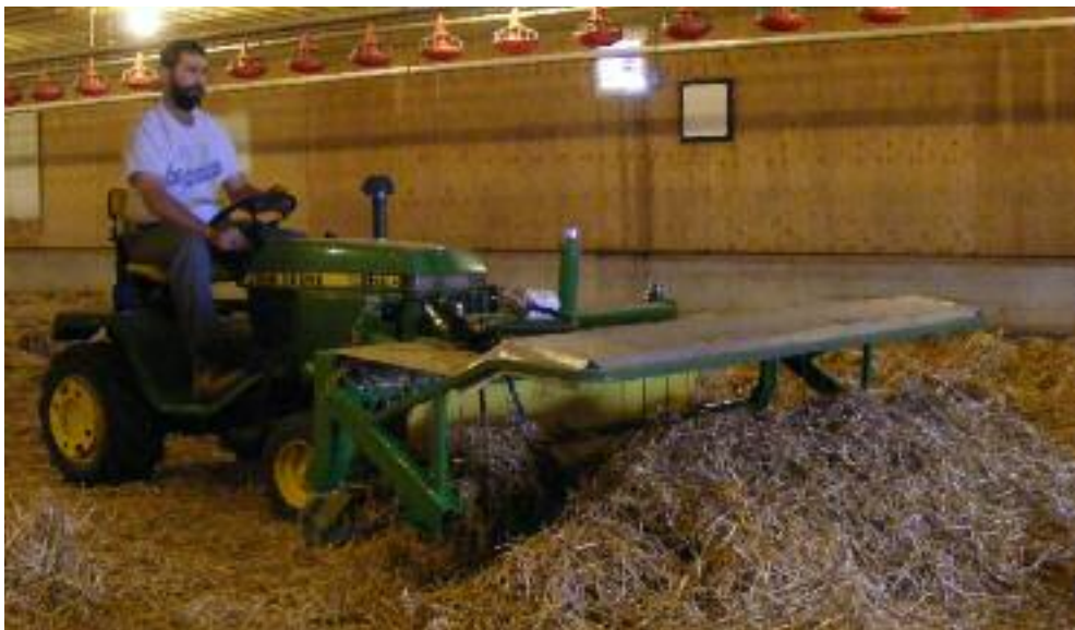
Rotary fork mounts on the push blades of most small utility tractors, making it easy to spread straw in poultry barns.
