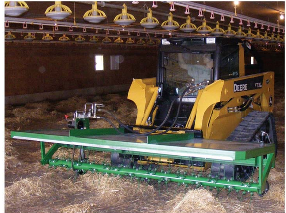
Hydraulic-operated rotary fork mounts on a skidsteer or tractor loader and is designed to evenly spread poultry bedding.
